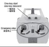
A. ONE-KEY START / ONE-KEY DESCEND: A: 一键启动/一键降落: s"ONE-KEY START / ONE-KEY DESCEND" key to start the aircraft. This time notor of the aircraft will be running slowly. Push upward the throttle leaver,the ircraft will take off "res"ONE-KEY START / ONE-KEY DESCEND" key during the course of flying,the ircraft will be landing slowly until landing on the ground and stop flying. . 按一下"一键启动/一键降落"键启动飞行器,此时飞行器马达将慢速动转,向上推油门
