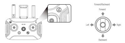
In GPS positioning mode, you can press the "One Key Return" button to return the aircraft. Do not control any functions during the process of return or ascent. When the aircraft is landing, you can toggle the joystick as to control it to land on your desired location. When the aircraft is returning to home point, long press the "Return" button to exit auto return mode.
