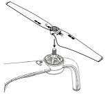
(1) Insert the CCW propeller into the shaft B (motor with concave points on the shaft end).
