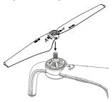
Insert the CW propeller into the shaft A (motor with concave points on the shaft end).
